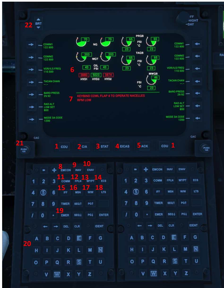
Figure: Center/Control Display Unit Page
